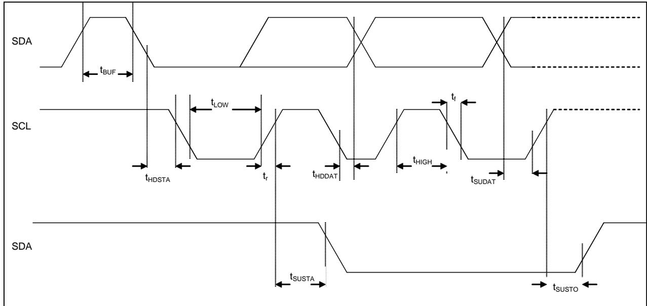
Figure 31: I<sup>2</sup>C timing diagram
