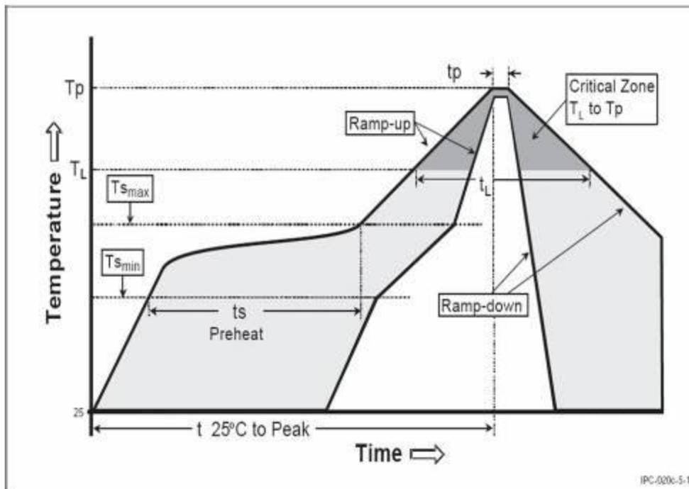
Figure 45: Soldering profile recommendation
