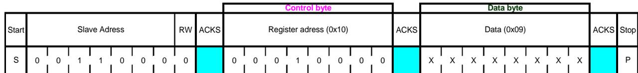
Figure 32: I<sup>2</sup>C write
