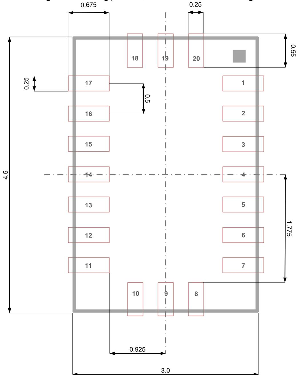
Figure 44: Landing patterns, dimensions are in mm
